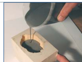
Casting a filled resin for a solid object
