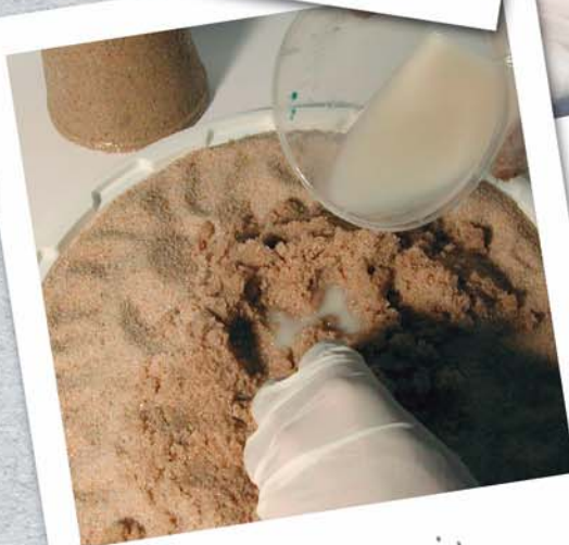
Preparing a resin concrete: sand + PU
