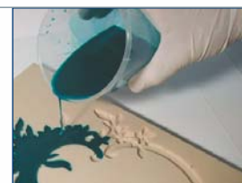
Tinted PU resin gravity casting
