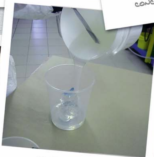
Making a mold in Essil silicone for parts in epoxy resin PX 521 HT
