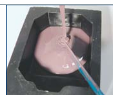
Casting of a filled epoxy resin
