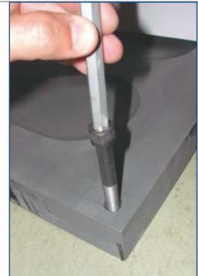
Threading in a tool in aluminium filled epoxy resin
