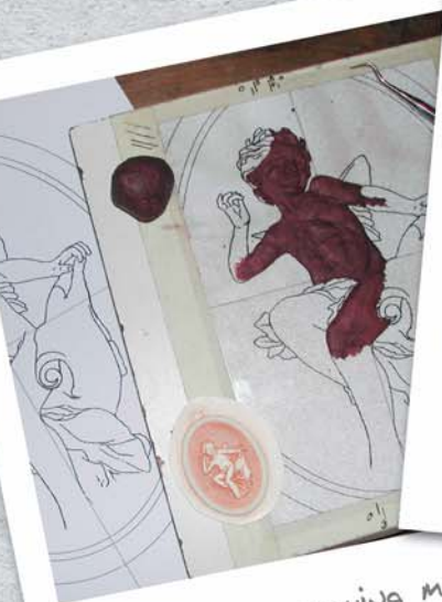
Making a mold in Essil silicone for parts in epoxy resin PX 521 HT
